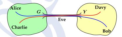
Suppose that the gateways G and Y link the green and the yellow LAN by an encrypted but *not authenticated* IPsec tunnel using a fixed SA. Assume that the encryption is done by some symmetric cipher in CBC mode. We want to show that Eve and her boss Davy can read all the traffic between Alice and Bob.
